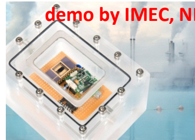
Low-ppb sensitivity for NO 2 GaN-based sensor concept
