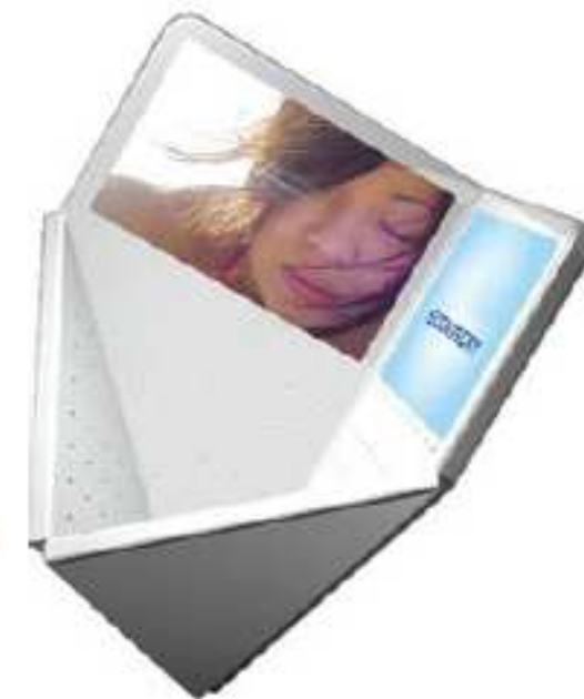
Nokia Scentsory Concept e-nose samples the odor of caller environment and transmit to recipient electronically
