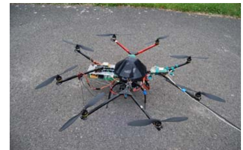
An Octocopter , the first platform on which we ( Max Planck Institute for Biogeochemistry, Jena, Germany ) tested a measurement sensor package for air quality sensors.
