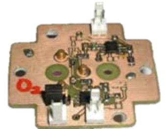
Alphasense: Electrochemical \text{O}_2 sensor
