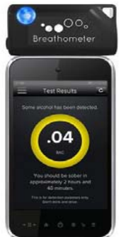
Plug-in modules or wireless monitors available (<$50) for smartphones display alcohol content from breath sample
