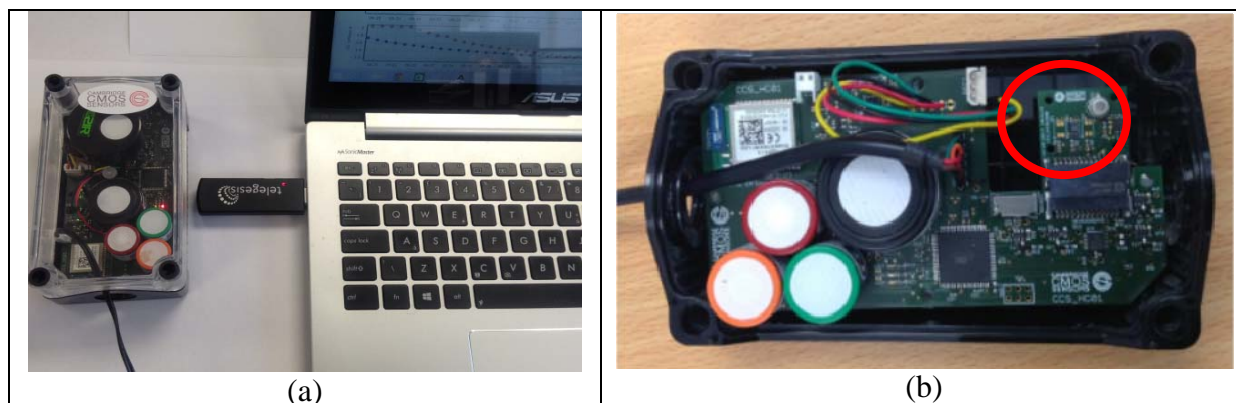
Figure 1. Example of sensor module: (a) Multi-parameter environmental sensing module; (b) Board with CMOS sensor modules providing same functionality (circled in red).
