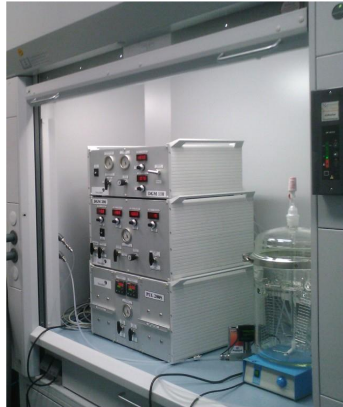
Generation of calibrated gas mixtures
