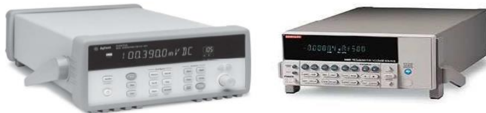
Agilent 34970A (~100M \Omega ) and Keithley 6487 picoammeter (~10 -16 \Omega )
