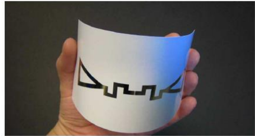
Photograph of the conformal tag with a SWCNT film in the center.
