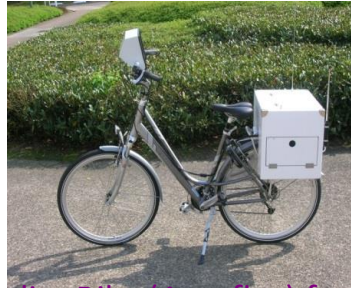
Air Quality Bike (Aeroflex) for Mobile Measurements by VITO, Belgium
