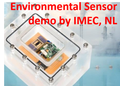
Low-ppb sensitivity for NO 2 GaN-based sensor concept
