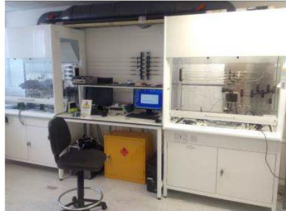
Gas test systems with MFC and fully automated control software
