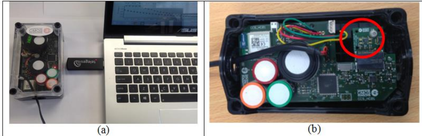
Figure 1. Example of sensor module: (a) Multi-parameter environmental sensing module; (b) Board with CMOS sensor modules providing same functionality (circled in red).]
