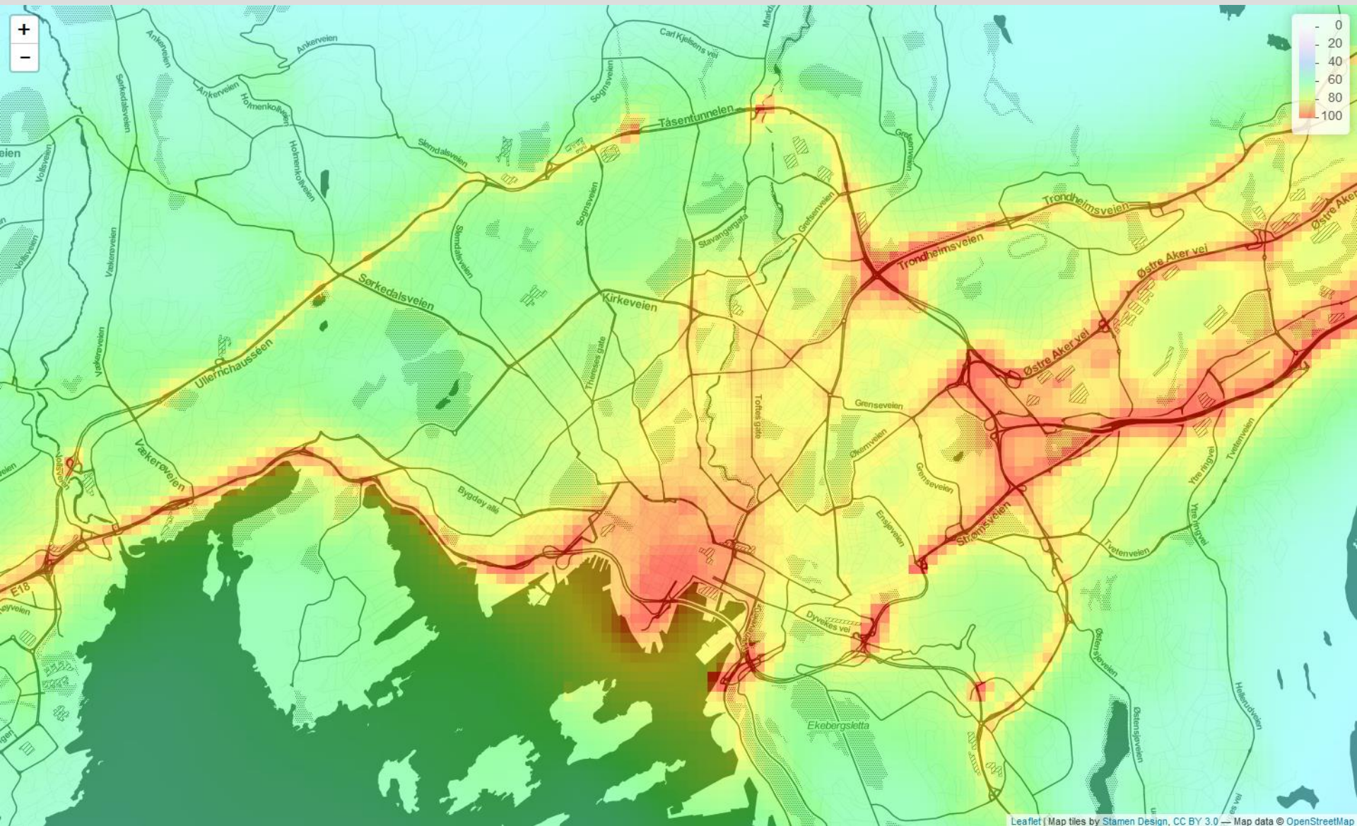
Typical example of a data fusion-based surface concentration field of NO 2 for Oslo, Norway, at 100 m spatial resolution.
