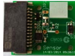
Fig 3: Daughter board with multi-gas sensor
