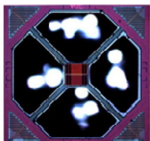
Figure 1: Microhotplate with \text{SnO}_2 - Au sensing layers (ams)
