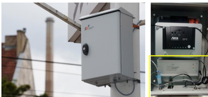
Figure 1. Weather proof housing (left) and inner workings (right) with measuring box (right, framed).
