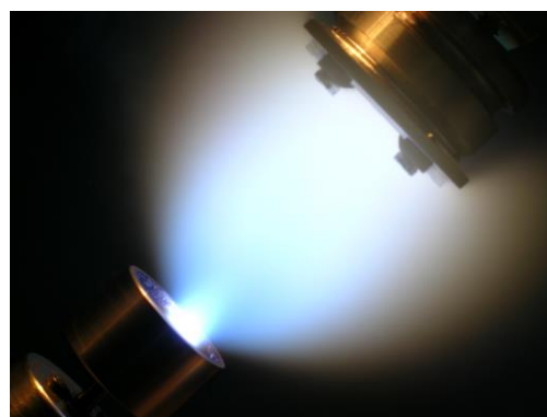
Figure 1. (a) Quartz crystal microbalance (QCM) measurements of PLD process of \text{WO}_3 revealed two modes of growth: (i) thin-film growth in the pressures p(\text{O}_2) \leq 0.05 mbar, and (ii) nanoparticle formation in the higher oxygen pressures. (b) With higher p(\text{O}_2) values ablation plasma starts to glow bright blue.
