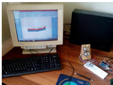
Figure 1. Sharp PM 2.5 sensors connected on Arduino platforms (S1 and S3 on the left, S2 on the right)
