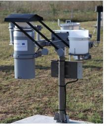
WADOS: Wet and dry only deposition sampler
