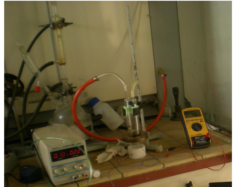
(A) Scheme of the setup used for the measurement of the concentration of methane dissolved in water. (B) Photo of the setup used for the measurement of the concentration of methane dissolved in water.
