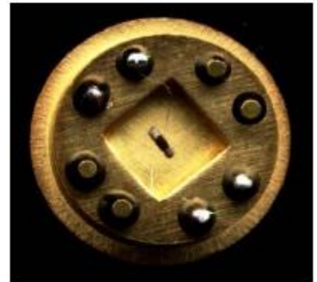
TO-8 packaged thick film sensor chip. Chip size 2.5 x 0.3 x 0.1mm
