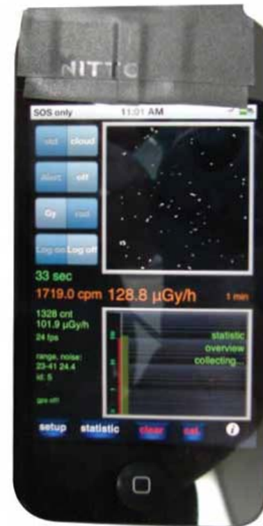
iPhone 4s using camera covered with black tape & SW app 1 \mu\text{Sv/h} (min) Source: ansto (2014)
