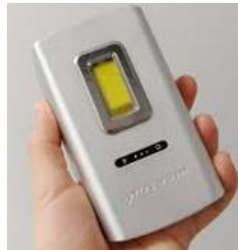
Low-cost ATR spectrometer for liquid
