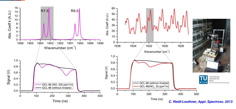
pulsed chirping-mode QCL operation scans across band Alternative: external cavity QCL with scanning mirror
