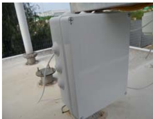
Figure 5. NASUS sensor system integrated in box (IP65/66) for Air Quality Monitoring in sensor networks at outdoor level.
