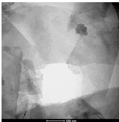
FIG. 1. TEM image of the flakes produced by chemically exfoliated graphene. The mean lateral size of flake is of the order of hundred nanometer.
