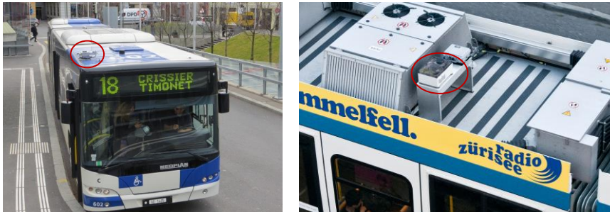
Figure 1. OpenSense sensor nodes on top of t-1 bus in Lausanne (left) and VBZ streetcar in Zürich (right)
